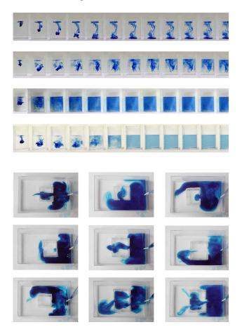
Figure 5. Emilie Tennant and Carin Nakanishi tested the impact of physical obstruction on flow. These tests share a lineage with both Victor Olgyay's wind/smoke studies as well as physical models chronicled in On the Water: Palisade Bay (see endnote 15). The physical model allows for simple empirical tests for understanding fluid behaviors.
